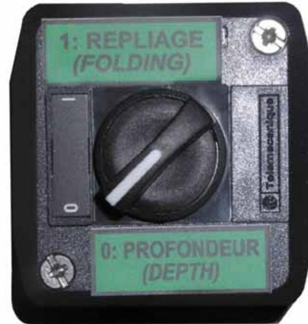
Turn selector to choose desired hydraulically controlled function
