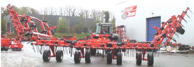
Eurocult 5 000 range 1st phase of folding cycle external lateral frames or outer wings
